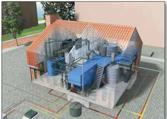
Noorderhoek, Sneek, (NL) "Waterschoon" project, local wastewater treatment for 230 houses
